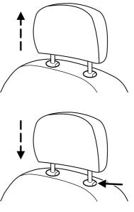
Properly adjust the head restraint so that the top of the head restraint is even with the top of your head and positioned as close as possible to the back of your head. For occupants of extremely tall stature, adjust the head restraint to its full up position.
